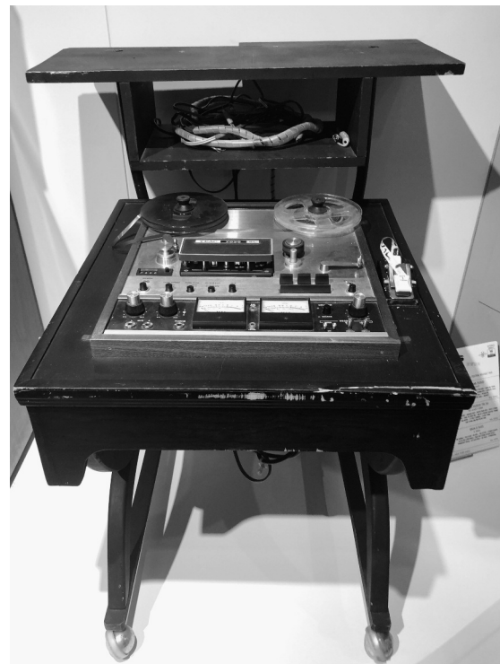
Hi Records tape machine. TEAC 7030 reel to reel which recorded such stars as Al Green, Ann Peebles, and O.V. Wright at Willie Mitchell's Royal Studios. Photograph by LaDawn Lee Fuhr.
